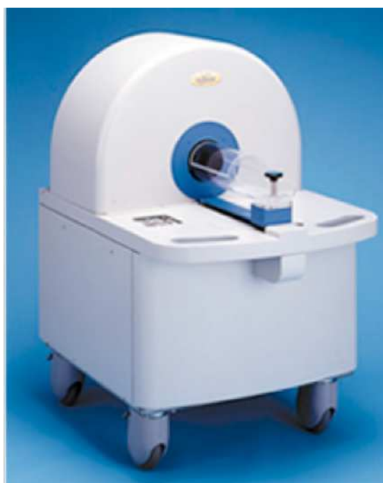
Fig.3-3 X-ray computed tomograph imaging system. X-ray CT imaging of rats was performed using LCT-100 type manufactured by Hitachi-Aloka Medical Co., Ltd.
