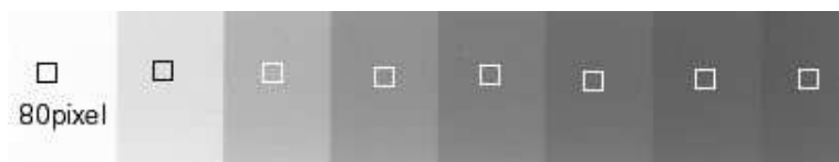
Fig.5-4 Aluminum staircase stage used as image density control. The density calibration, using an aluminum stage as a reference. In order from the thinner of the concentration, an average pixel value of an image contained in a square area of 80 \times 80 pixel measured at each stage of the aluminum stage.
