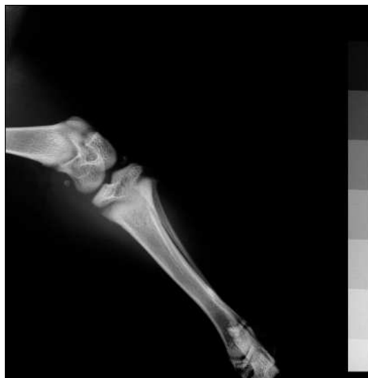
Fig.4-5 Image with density calibration using IP Lab which is image analysis software.
