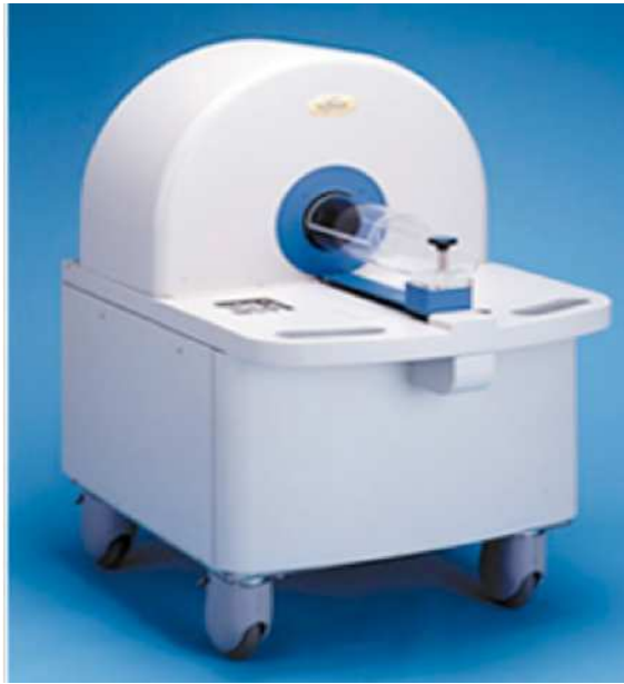
Fig.5-21 X-ray computed tomograph imaging system. X-ray CT imaging of rats was performed using LCT-100 type manufactured by Hitachi-Aloka Medical Co., Ltd.
